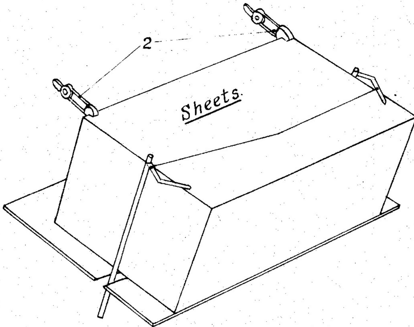
down onto the eccentric stud on the connecting bracket and lock up the claw in that position. Release the locking bar again and pull the feeder away from the machine. Tighten up eccentric stud on left-hand side. Repeat this whole operation from 14 with the right-hand claw.
