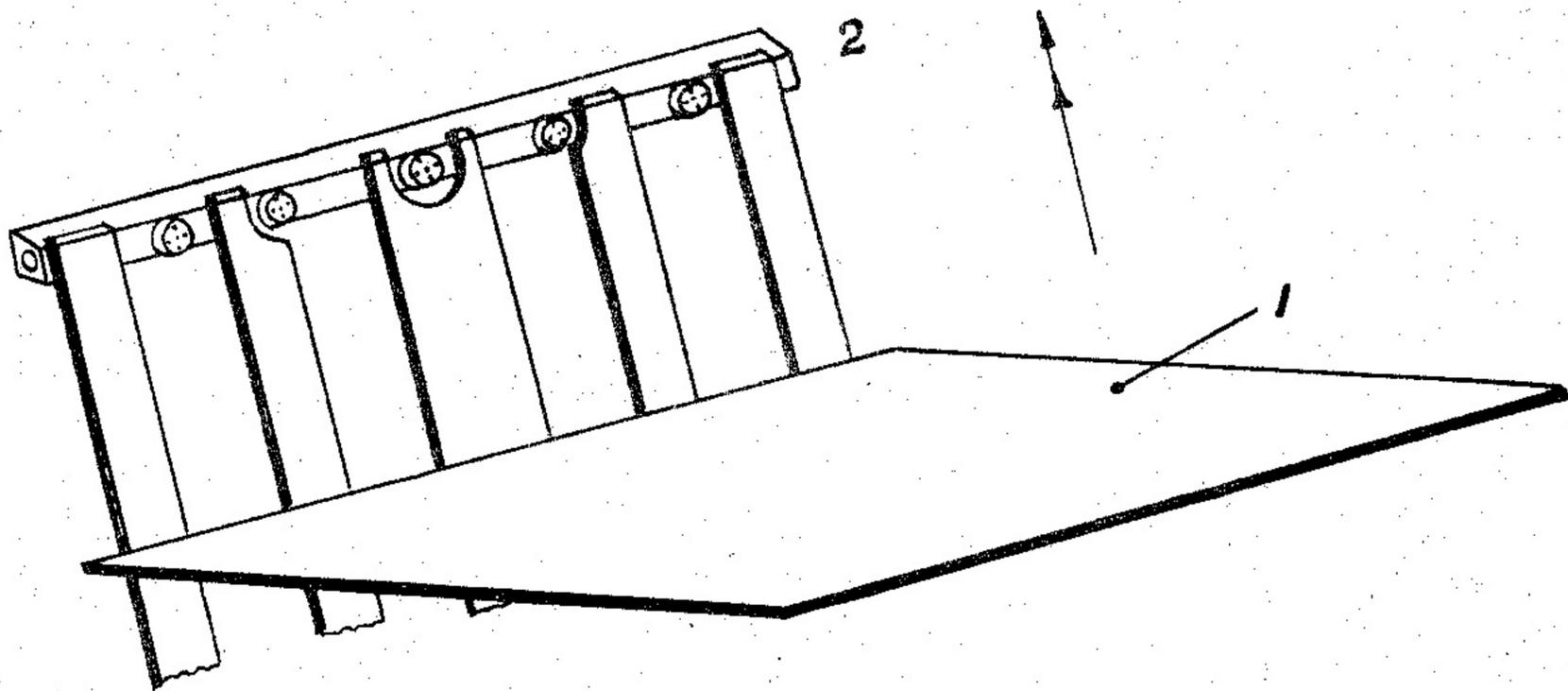
Then from the back of the feeder, push the locking bar down onto the eccentric stud on the connecting bracket and lock up the claw in that position. Release the locking bar again and pull the feeder away from the machine. Tighten
