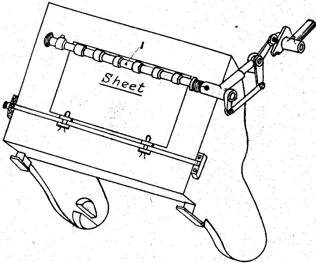
Then from the back of the feeder, push the left-hand claw down onto the eccentric stud on the connecting bracket and lock
