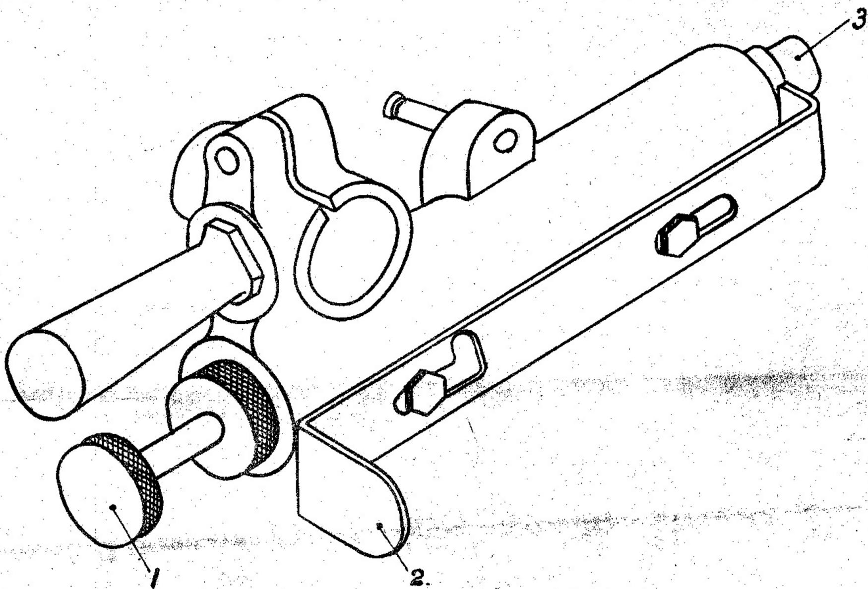
From the back of the feeder, push the left-hand claw down onto the eccentric stud on the connecting bracket and lock up the claw in that position. Release the locking bar again and pull the feeder away from the machine. Tighten up eccentric stud on left-hand side. Repeat this whole operation from 14 with the
