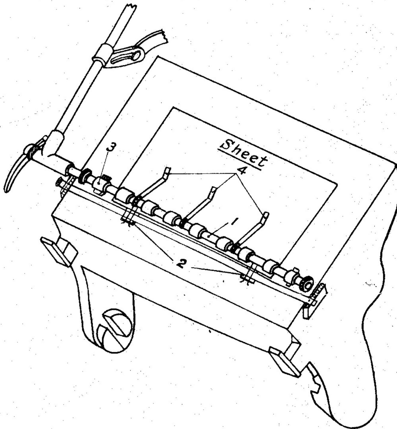
From the back of the feeder, push the left-hand claw down onto the eccentric stud on the connecting bracket and lock up the claw in that position. Release the locking bar again and
