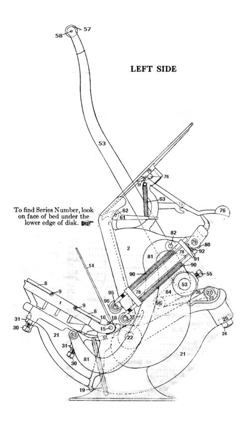
Remember the right side of the press is the left-hand side of the operator, if he stands facing the press. If the left-hand side is ordered it will be understood as the right side of the machine itself as it faces the operator.
