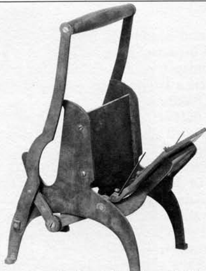
Fig. 6. Prototype of the famous Pearl Press. This is the patent model submitted by W.H. Golding. (U.S. Patent no. 145101, 2 December 1873.) (Courtesy Smithsonian Institution and Elizabeth Harris, Curator, Graphic Arts Division.)
